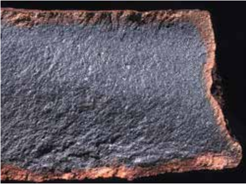
Figure 7. Weathering 'skin' about 1 cm thick surrounds fresh, hard, fine-grained granophyre. The outer 1 mm comprises mainly iron oxides precipitated along former joint planes or accreted in the surficial environment from wind-blown material and/or organic activity, and the paler brown material beneath the outer rim is largely kaolinitic clays formed by break-down of feldspars, iron oxides and hydroxides formed by weathering of pyroxene, and fine grained quartz which is essentially impervious to the weathering process.
