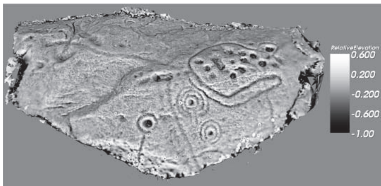
Figure 7. Perspective view of the Horseshoe Rock 3D model coloured corresponding to relative elevation after high-pass frequency filtering. The small black spots with surrounding white halo are due to outliers in the data.
