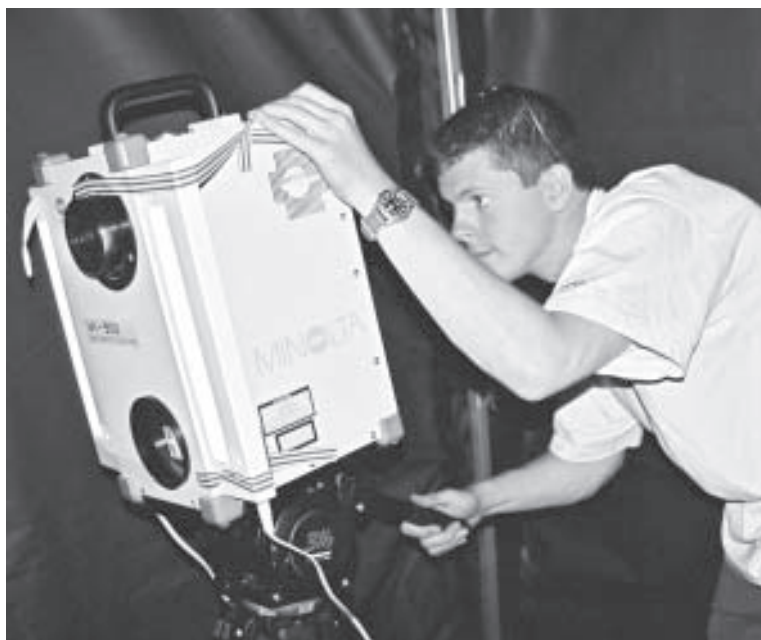
Figure 1. Photograph showing the Minolta laser scanner used for the recording of the data presented in this article. The portable operated scanner was placed under a tent in order to exclude interference from external light sources.
