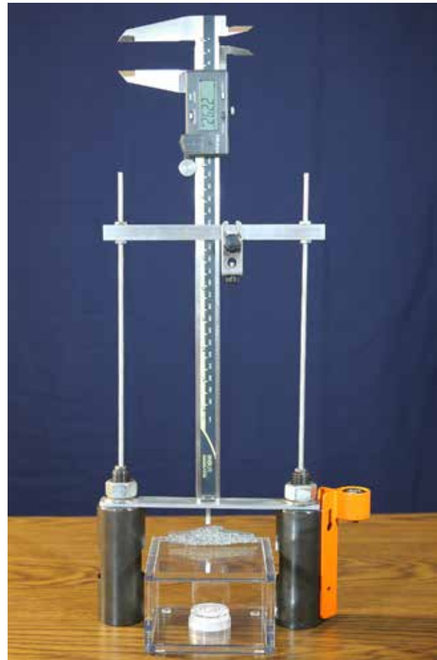
Figure 1. Microtopography system model MT1. Measures 20" high with a 12" long calliper, 9" wide and weights 5 lb. The height can be reduced to 14" with a 6" main scale long calliper. Note the bull eye (white) and vertical (orange) levels. Photo and diagram by JC.
