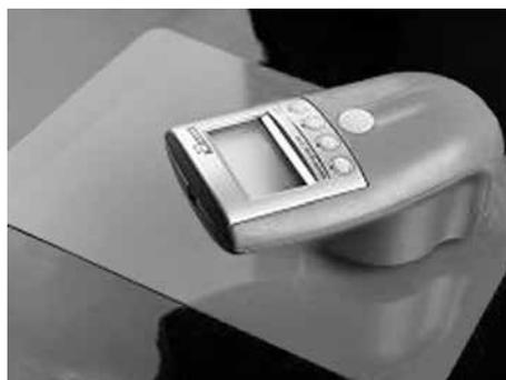
Figure 1. The BYK-Gardner model 45/0 portable spectrophotometer used in the study by Lau et al. (2007).
