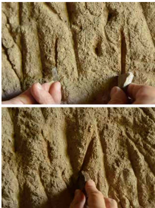
Figure 6. Experiments of incising Guadalupe Tuff: glass and siltstone (left to right, upper); and chert (lower). Source AJ.
