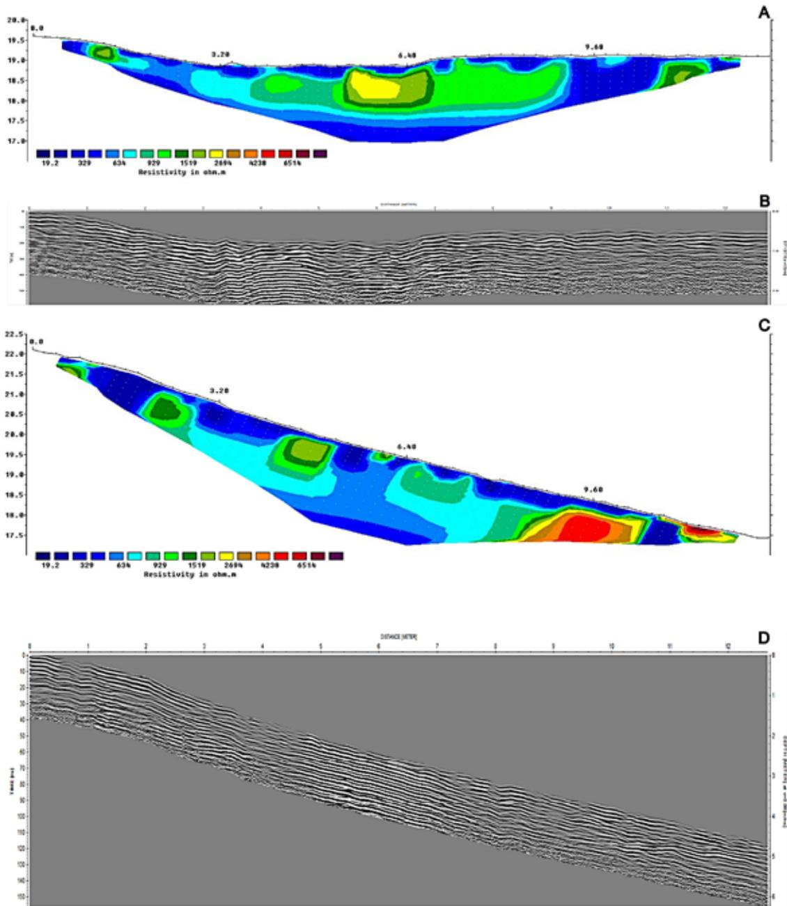
**Figure 7.** Geophysical data from the Thurk Petroglyph Site. Line one data for ERT (A) and GPR (B) is displayed from the north-east (left) to the south-west (right). Line two data for ERT (C) and GPR (D) is displayed from the north-west (left) to the south-east (right). Distance along the line is in metres and elevation is provided in AHD for the ERT data and in relative values for GPR data.
